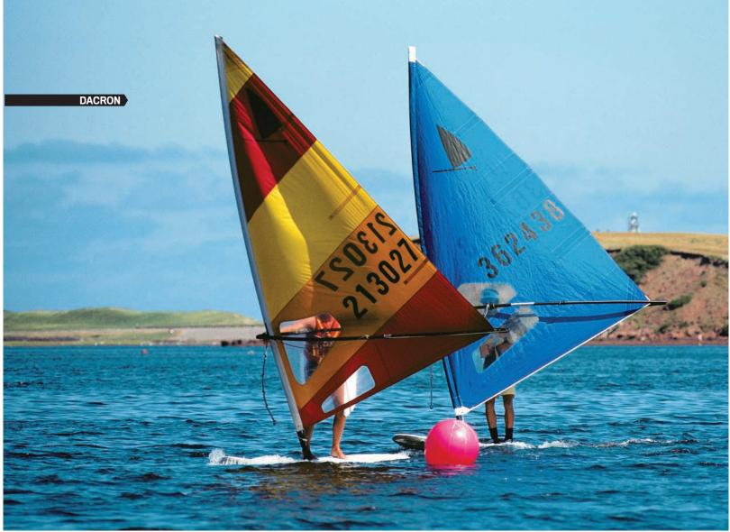
Dacron is what sailmakers were using for sailboats in 1968, when Hoyle Schweitzer built the first Windsurfer, so that's what was used. The woven polyester blend made by DuPont worked - pretty well, in fact. It kept working for 12 years, with the basic design of the original Windsurfer sail changing very little as the sport grew. But the Dacron of that era had its disadvantages - it was soft and prone to stretching over time.
